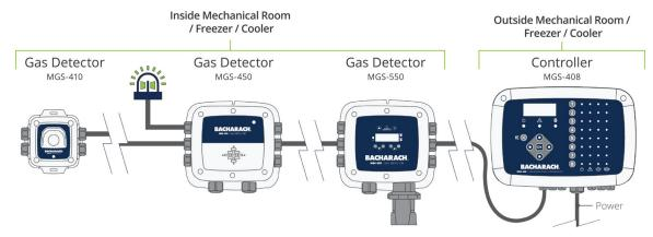
Figure 1. Power Cable Application
