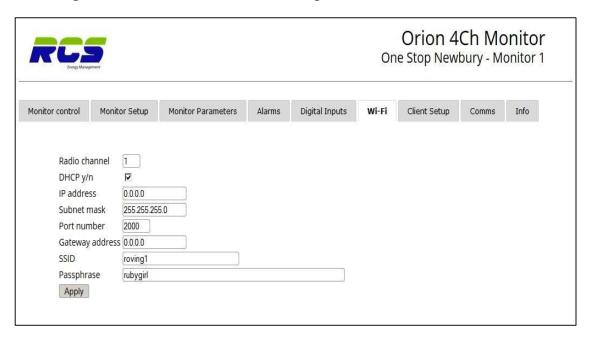
If the unit purchased is a standard (wired) Ethernet version (Not Wi-Fi) then the Wi-Fi page of the configuration will NOT be displayed. as per Fig 9 above, Otherwise the following parameters are available. Please refer to your network administrator if unsure of any settings.
