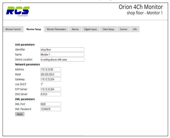
The second tab is "Monitor Setup" (Fig 2) containing the following options / information:-
